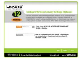
Figure 7-17: Configure Wireless Security Settings - WPA2-PSK Screen
